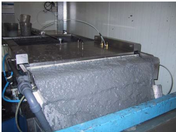
conventional surface skimmer paint sludge with high residual moisture
