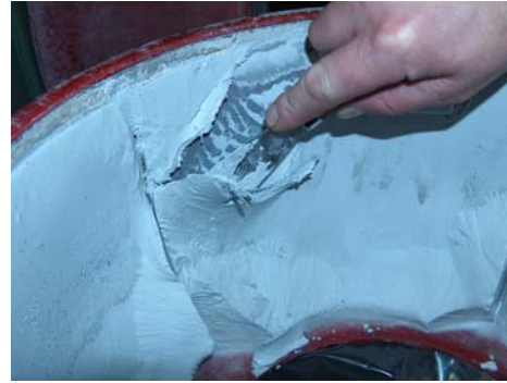
separated glass sludge from STA centrifuge – compact and dry cake solids
