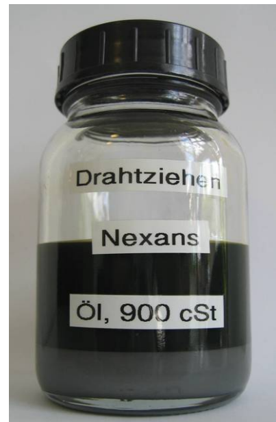
Picture #1: A Sample of polluted drawing oil after 9 months; only after a very long period the particles settle completely
