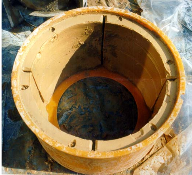
Sludge insert from the centrifugal separator, filled with cake dry phosphate sludge
